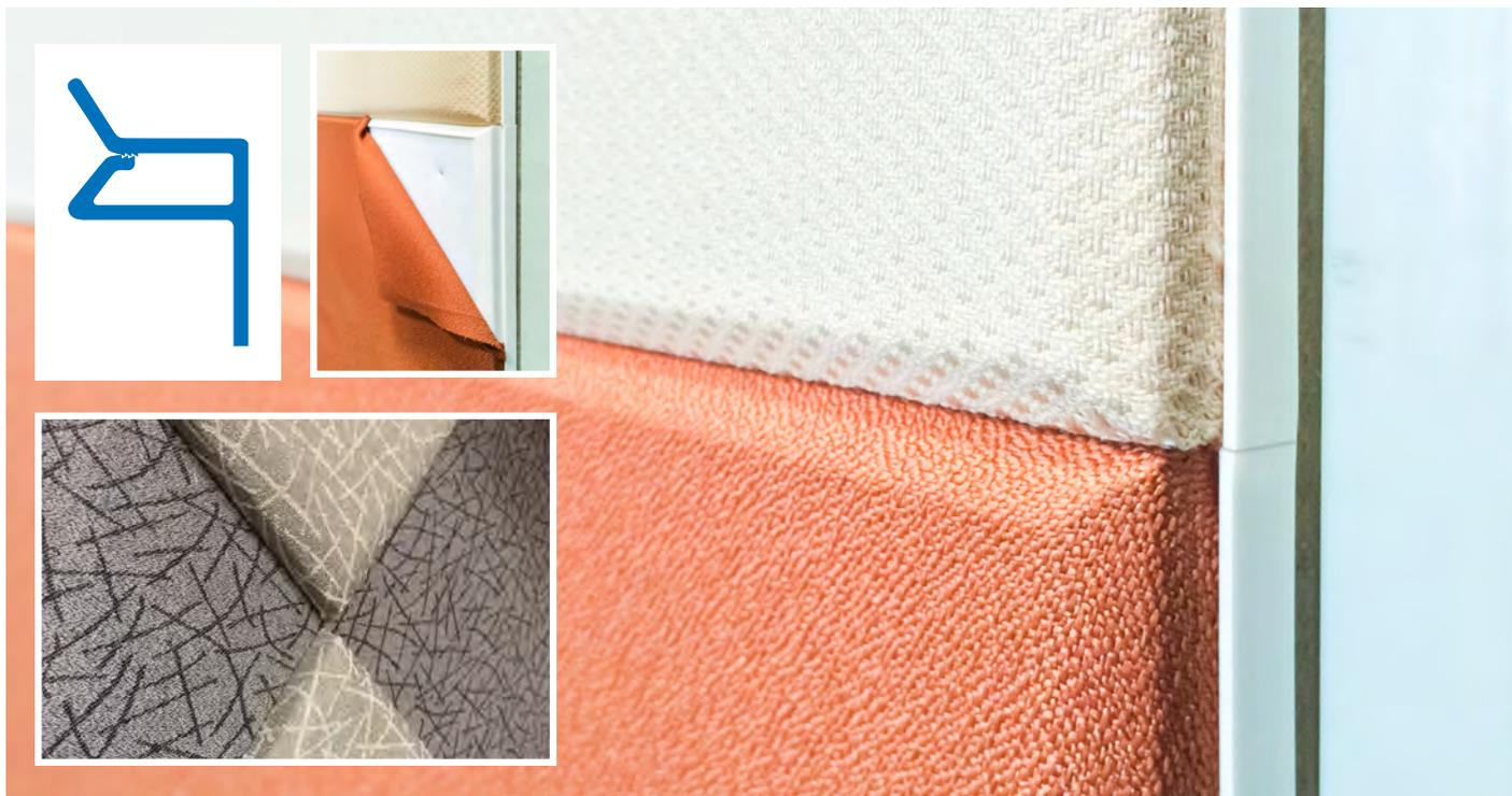
FS280 is used as a beveled intermediate piece to join two sections of paneling for 1" thick wall finishing installations. Available in a natural color. Pantone Match Color Available. (Lead times & minimum quantities apply)
